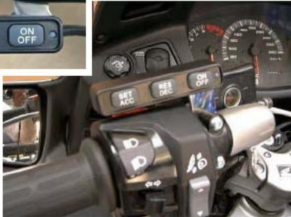
The cruise control uses an electronic "computer" module to maintain any required speed between 25 and 100mph (40-160kph) according to model.
