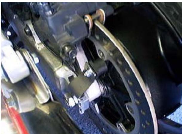
The **Speed Sensor (7)** is mounted on the left hand side of the swing arm on the rear axle. Nickel plated magnets are placed in the heads of the bolts that mount the brake disc.
