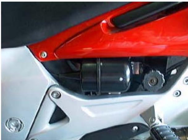
The **Vacuum Actuator (3)** (throttle servo) is mounted on the left side of the bike next to the bike's rear suspension preload adjuster. Aluminium covers finished in satin black powder coat are provided to protect the actuator and enhance its appearance. The actuator mounting bracket incorporates a new mount for the preload adjuster. A **vacuum hose assembly (4)** is provided to connect the actuator to the engine.
